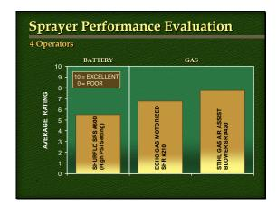
Data as the average from 4 experienced operators evaluating a selection of **motorized** sprayers "in field" representing small-scale farming. Operators were instructed to provide a **single evaluation number from 0 to 10 with zero being the poorest and 10 being the best**. They considered primarily application
