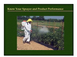
A modern lightweight motorized sprayer is capable of delivering spray pressures in excess of 100 psi. If agricultural spray products require very fine misting droplets and the crop has large amounts of leaf area a motorized sprayer either hydraulic or air assisted may be a better choice than hand operated backpack sprayers.
