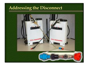
Two sprayers represent, on right a factory original sprayer - on left a sprayer adapted to Spraying Systems – TeeJet spray handle components including a CF pressure regulating valve, quick change nozzle body, strainer, rubber gasket, turbo flood jet nozzle, and snap lock nozzle cap.
