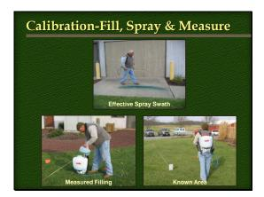
This slide shows the three steps of a simple calibration method [Fill-Spray – Measure]. First determine the spray Width of nozzle, add a known amount of water to the sprayer, flag a known area at the proper nozzle spacing, then spray area, then measure how much spray solution was utilized for the known area. For example measure a 1000 ft.² and determine ounces of spray material required. It's important to walk at a constant speed and maintain nozzle height to provide the appropriate coverage.
