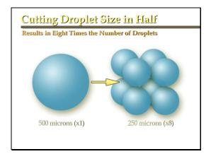
A basic spraying principle - changes in droplet size dramatically increase or decrease leaf coverage with the same quantity of water. Since backpack sprayers have limited capacity this is an important concept especially with products requiring good leaf coverage. However smaller droplets drift more.
