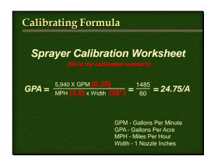
Gallons per Acre is a common calibration measurement for applying agricultural products. Formula represents a simple calibration method requiring three measurements. 1] flow of nozzle in gallons per minute, 2] constant speed in miles per hour and 3] constant spray width. The operator of backpack sprayers should calculate speed in the field not in a driveway, a pressure regulator is helpful to calibrate gallons per minute and holding a constant nozzle position maintains a constant spray width.
