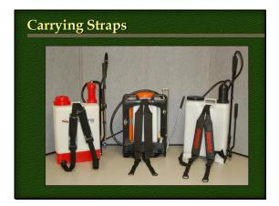
Backpack sprayer's filled with spray solution weigh 30 to 40 pounds. A comfortable and convenient carrying system is important to ensure operator comfort, reducing fatigue which enhances application practices.
