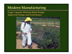
A video clip of a well-designed handoperated backpack sprayer: notice operator pumping at a comfortable rate due to efficient, high capacity internally mounted piston pump with appropriate nozzle, sized for sprayer as well as pest control products requirements.
