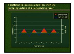
Hand pump sprayer's fluctuate in pressure with up-and-down pump strokes as noted in this slide causing uneven flow rate and poor calibration. Adding a pressure regulator ensures constant flow rate an important calibration criteria. The following slide discusses pressure regulators.
