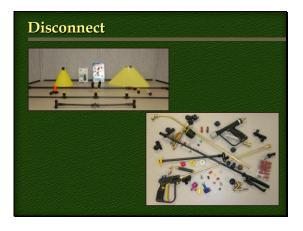
The "disconnect" refers to - need to combine sprayer with a wide selection of application components such as nozzles, strainers, pressure regulators, multinozzle assemblies etc. addressing application requirements of the multitude of liquid products small-scale farmers apply such as; compost teas, clay suspensions, emulsions etc.
