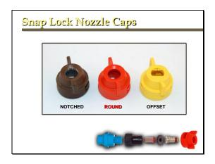
Point out that there are many different styles of nozzle caps which are specifically designed for various nozzles but they are related to multi-nozzle boom sprayers. For backpack sprayers utilizing a single nozzle the Round nozzle cap should always be used. The reason is that it allows the nozzle to be freely rotated to align the nozzle based on operators requirements. The other nozzle caps prevent the rotation of the nozzle.
