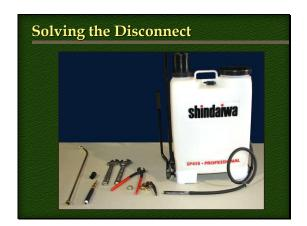
Retrofitting Spraying Systems – TeeJet spray handle assembly requires a few common tools and a few minutes – approximately \$100 in parts for conversion. The conversion allows the farmer access to all the compatible quick change nozzle bodies, nozzles, screens etc. from the manufacturer.
