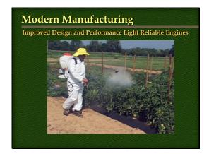
Video clip demonstrates modern lightweight gasoline powered backpack sprayer providing reliable performance. Note: these types of sprayers are most appropriate for higher pressure application 30 to 100 psi
