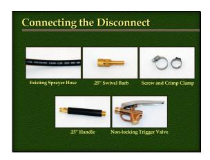
Conversion parts required for a Spraying Systems – TeeJet assembly –swivel barb is recommended preventing operator fatigue from spray hose twisting— a non-locking trigger valve is recommended to prevent accidental application from the trigger valve failing to shut off due to locking mechanism – either hose clamp works but the crimp clamp works better preventing leaks and not catching clothing.
