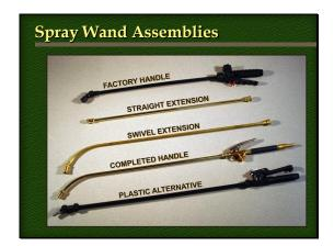
Various spray handles displayed below the original factory handle of a Solo sprayer provide insight into the flexibility attained converting sprayers to a Spraying Systems – TeeJet handle assembly – various length extensions addressing operator and crop height variations are available. Curved, straight, swivel nozzle bodies, as well as plastic components allow for flexibility in application criteria.
