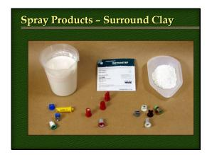
Surround WP [Wettable Powder] is utilized at high concentrations in water carrier potentially clogging nozzles. Inappropriate nozzle and strainer combinations as noted on green strainer[100 mesh] left is clogged making application problematic. Red strainer [50 mesh] in middle is working properly but still showing signs of potential clogging. The white strainer [25 mesh] shows no signs of clogging. Nozzle orifice size must be slightly larger than the mesh size.
