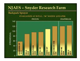
Evaluation data of hand-operated backpack sprayers representing piston and diaphragm pumps. The number of pump strokes per gallon of spray was determined for each sprayer utilizing a 30 psi pressure regulator and a nozzle producing 0.52 gallons per minute at 30 psi. The nozzle and operating pressure were selected to maximize pumping requirements. Sprayers were modified with a "Spraying Systems-TeeJet" handle assembly as shown in slide 20
