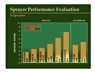
Data as the average from 4 experienced operators evaluating a selection of sprayers "in field" representing small-scale farming requirements. The operators were instructed to provide a single evaluation number from 0 to 10 with zero being the poorest and 10 being the best. They considered primarily application efficiency but also considered comfort, filling and clean out. Sprayers were modified with a "Spraying Systems- TeeJet" handle assembly and CF pressure regulating valve.
